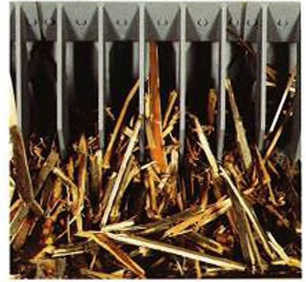
Picture 3: Waste wood preparation for coarse size-reduction in the slow-speed precrusher "Dracula"; material evacuation via conveyor belts and separation of the already set free ferritic parts by means of a magnet
