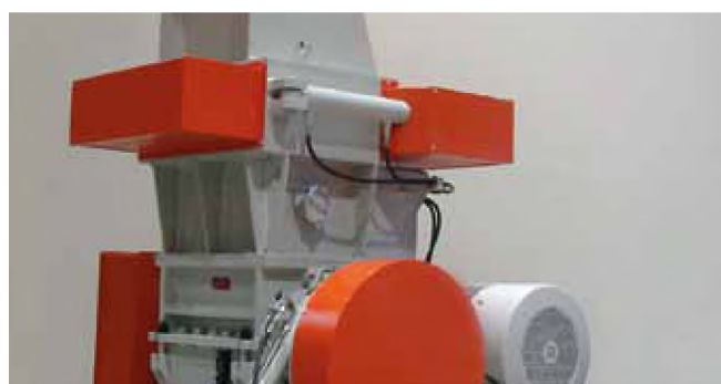
Bale cutter inserted into the infeed chute
